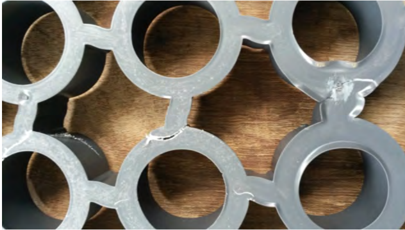
Figure 5 – Underside of sample tested with clear opening below, showing cracking of the sample
