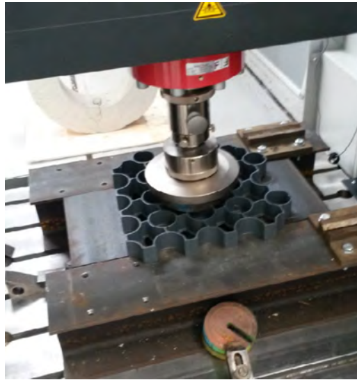
Figure 1 – Two-way 250 mm span test setup
