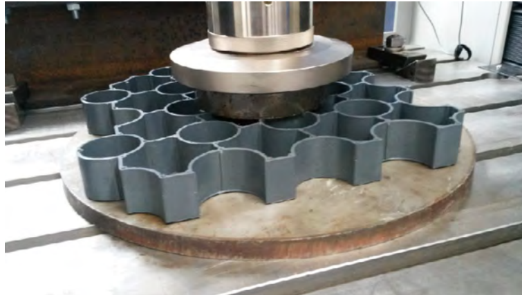
Figure 2 – Fully supported loading test setup
